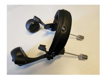
8. Connect the audio cable to the A2000 by bringing the magnetic connectors close to the magnetic sockets on the sides of the headphones. The connection via the sliding contact is made automatically by the magnetic attraction.
